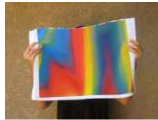
Lenticular polyester fabric can refract multiple different colors or images when moved.
