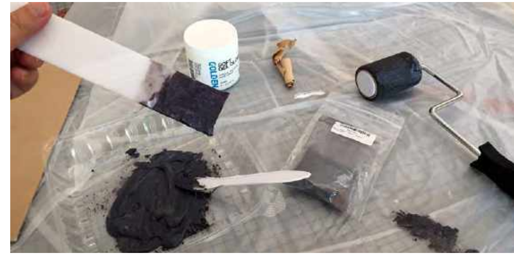
I mixed thermochromic pigments from Karlsson Robotics with a clear gel medium, then applied this mix to my design, which I had UV-printed on acrylic at RISD's Co-Works.
