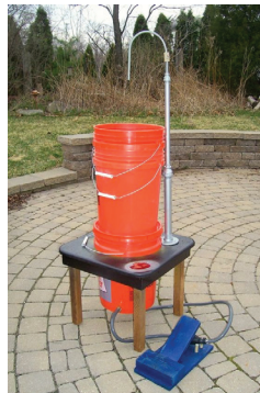
DIY Foot-pump handwashing Sanitary handwashing made of buckets, a foot pump, and scrap wood
