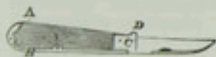
Pocket Knife 2592R-W4 A Scale; B Spring; C Tang of blade; D Kick
